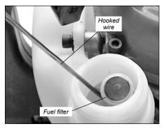
Before reinstalling the filter, inspect the fuel line. If you discover damage or deterioration, the unit should be removed from service unitl it can be inspected by a Shindaiwa-trained service technician.
